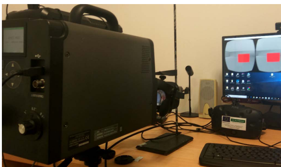
Figure 2: Experimental setup used for chromatic characterization of both HMD.
