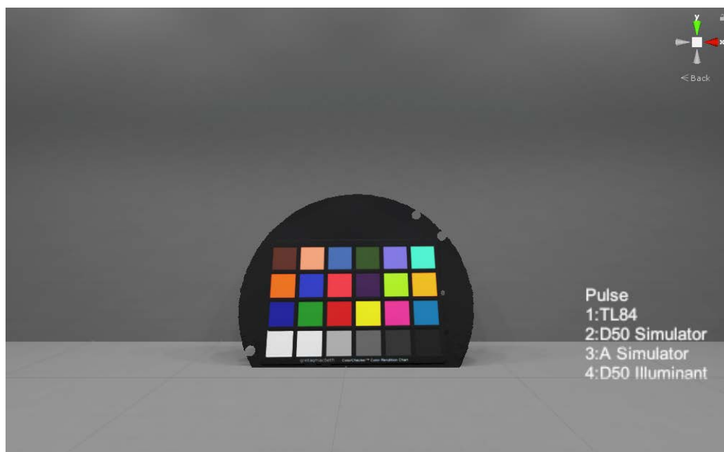
Figure 3: Virtual Light booth with colour checker calibration chart.
