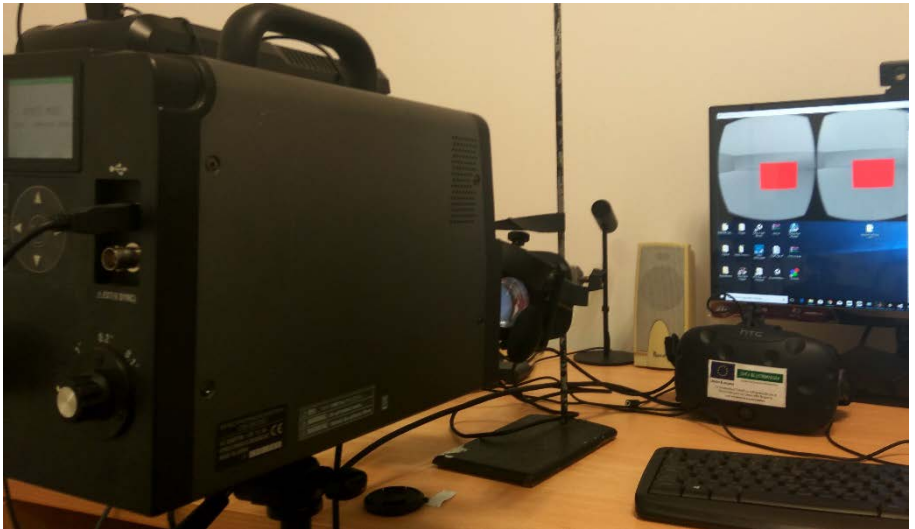
Fig. 3 – Experimental setup used for chromatic characterization of Oculus Rift Device.
