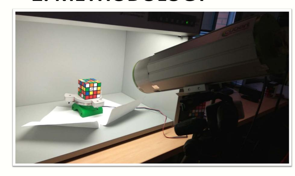
Scanning 3D objects and measuring the spectral reflectance with a hyperspectral camera and a telespectroradiometer, we can add spectral information to the 3D model to modify their color.
