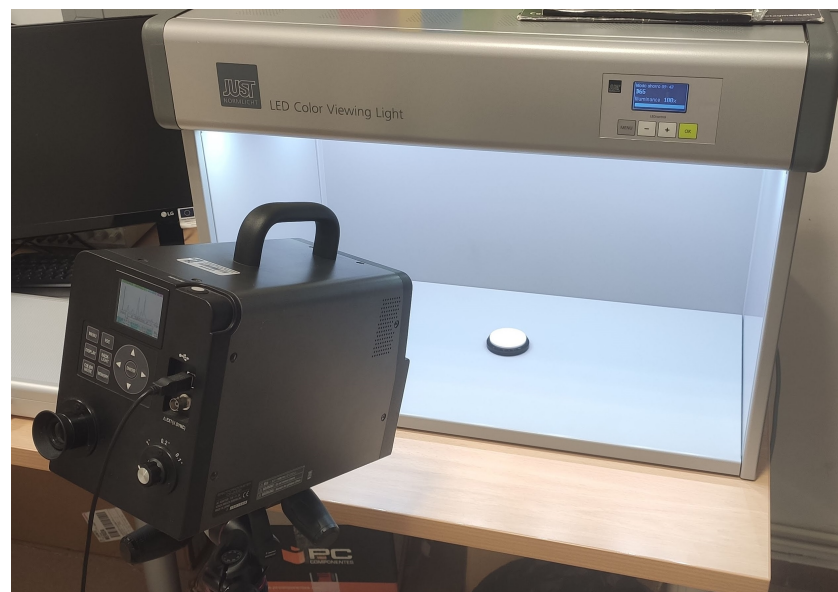
Figure 4. Set up of measurement of spectral power curves of real light sources.
