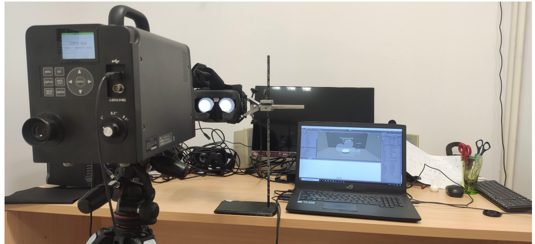
Figure 2. Experimental setup used for the chromatic characterization of the HTC Vive Device.
